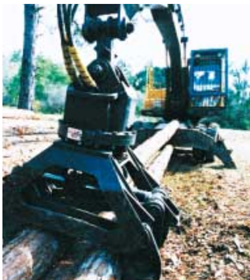
Left The Volvo excavator is fitted with wheels, which provide excellent travel speed and mobility, without affecting productivity.
